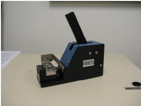
South Bay Model 310 3mm Disc Punch - for metals and alloys
