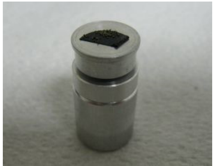
SEM powder sample stuck to SEM stub using a carbon sticky dot
