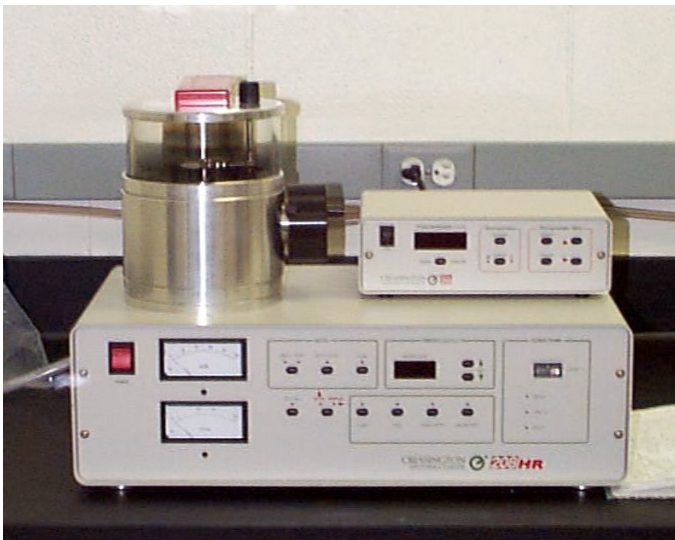
Cressington Sputter Coater used to coat non conducting specimens with Pt/Pd or Cr
