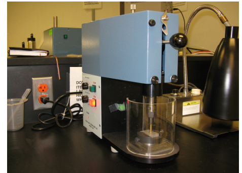
South Bay Model 360 3mm Slurry Cutter - for general purpose cutting
