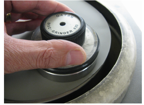
Disc grinder on a silicon carbide covered wheel. The amount of material removed can be set using the micrometer which moves the specimen and stub relative to the bottom face
