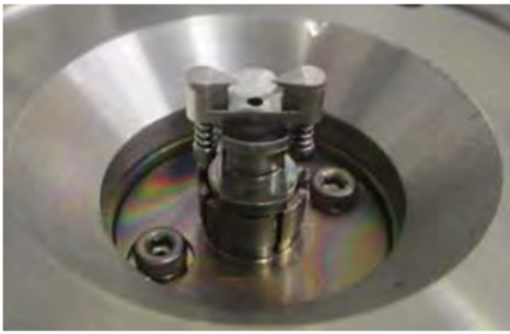
Specimen is clamped between two jaws before being loaded into the ion mill
