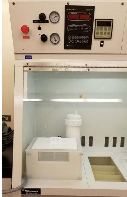
Potassium Hydroxide (KOH) etching is a wet chemical etching process used to create cavities in silicon. Highly corrosive alkaline chemical compound ( $\text{pH} > 12$ ) is used in conjunction with DI water and thermal regulation. The etch rate is depending on the concentration of the KOH solution and temperature. KOH is a strong, corrosive base and should be handled with extreme care.
