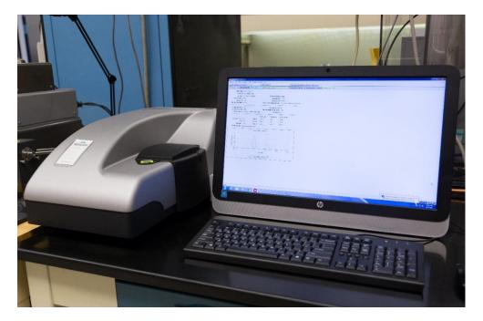
Dynamic light scattering is a well-established technique for measuring the size, Zeta potential and molecular weight typically in the range of 0.3nm (using highest technology) -  $10\mu$ m. Light scattering is a consequence of the interaction of light with the electric field of a small particle or molecule.
