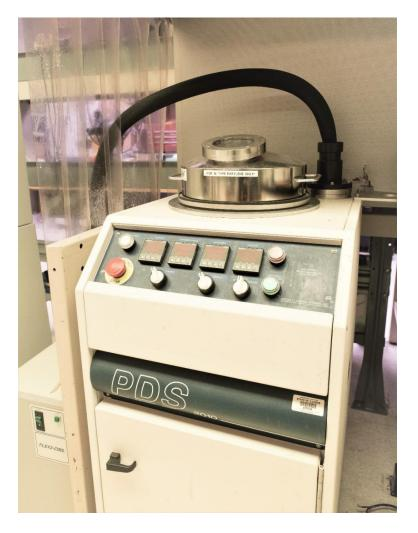
The Labcoater PDS 2010 is a vacuum system used for vapor deposition of Parylene C onto different surfaces. The very thin coating of the polymer provides a very effective chemical and moisture barrier, with high mechanical stability and dielectric constant.
