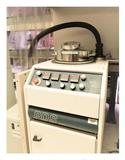
The Labcoater PDS 2010 is a vacuum system used for vapor deposition of Parylene N onto different surfaces. The very thin coating of the polymer provides a very effective chemical and moisture barrier, with high mechanical stability and dielectric constant.
