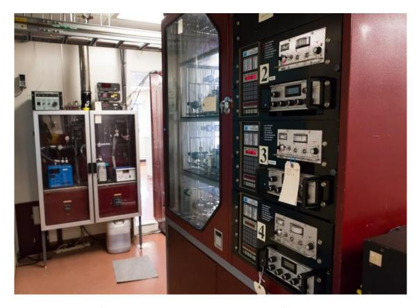
The PTL LPCVD system features 3 zone tubes that can be used for low and elevated temperature wafer processing. The system currently has 2 operations tubes. Tube 2 is used for undoped Polysilicon and low temperature oxides. Tube 3 is used to for Silicon Nitride deposition only. After passing the NCF safety exam, users can request training on this machine by sending an email to ncftech@uic.edu. Those not trained can request an NCF work service order by contacting the lab manager.
