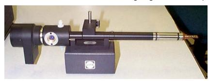
C additional water cooling is necessary. The temperature is reached within 1 minute and after 10 minutes drift rates should be less than 0.2nm/second. The maximum tilt for this stage is 8 degrees in X and 6 degrees in Y. Standard 3mm
