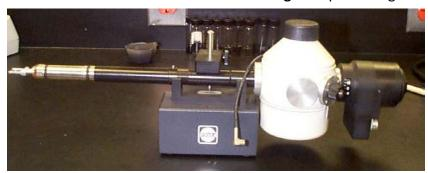
temperature of -170 deg C. Thermal drift after 45 minutes is less than 0.1nm/second. The maximum tilt for this stage is 18 degrees. Standard 3mm specimens fit in this holder.
