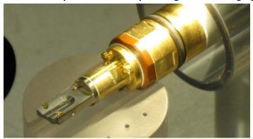
self-contained and fully hydrated flowing and mixing chamber, directly within the TEM. (Purchased by Tolou Shokuhfar)
