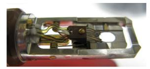
thermal E-chips or, provide a platform for precise electrical current and voltage biasing using Electrical E-chips. The specimen is mounted on an E-chip specimen support, which allows heating ramp rates of up to 1000 deg C per millisecond with ultra-low drift. The specimen volume must be kept to a minimum.
