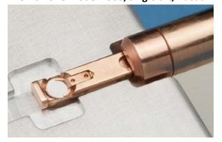
transferred to the microscope without seeing atmosphere. For specimen protection during transfer to the TEM, the specimen is retracted into the body of the holder, which in turn seals and isolates the specimen from the surrounding atmosphere. The holder is ideal for sensitive specimens that can be altered by environmental conditions; the specimen can be transferred in the presence of vacuum or an inert gas environment. Loading TEM specimens in
