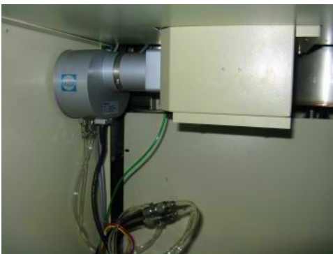
The new Model 830 Orius SC200 CCD camera is a retractable CCD camera capable of working at TV rate and slow scan replacing both of the previous cameras.
