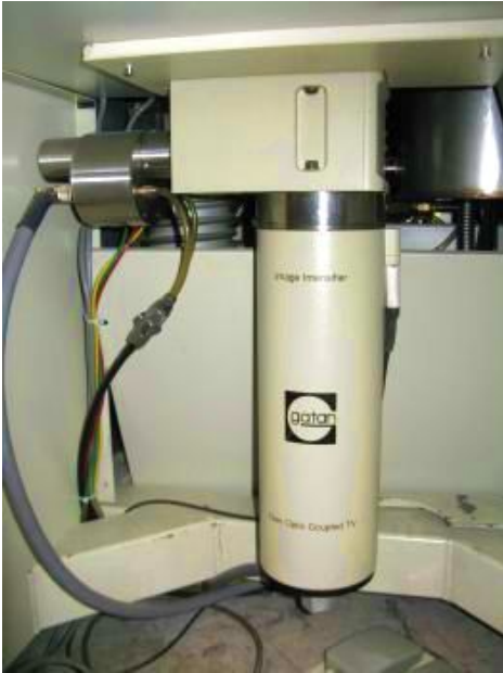
The old two camera system with the side mounted Model 694 1k x 1k retractable slow scan camera and the vertically mounted Model 622 intensified TV rate camera (8th March 2013)
